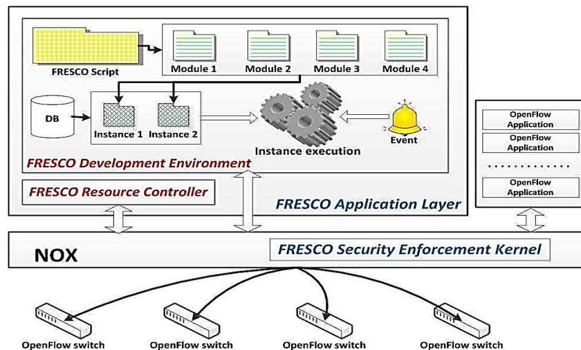
Fig. 3: High level overview of the FRESKO architecture [2].
