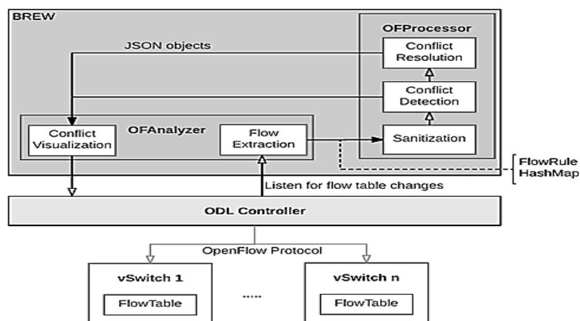
Fig. 4: System architecture showing Brew solution models [9].
