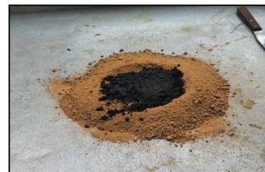
Fig 7: Preparation of geopolymer mixed with laterite soil.
