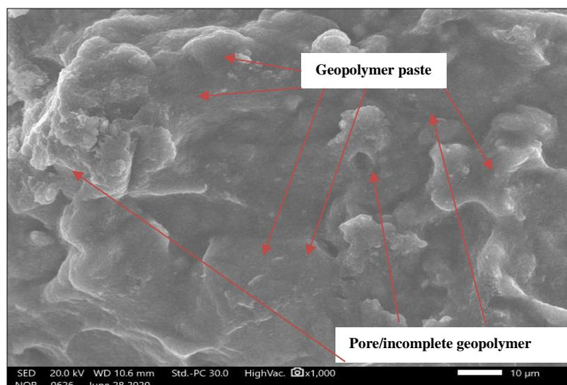
Fig. 14: SEM Samples of Laterite soil with 15% of Geopolymer (LS.15.0 GPOBA).
