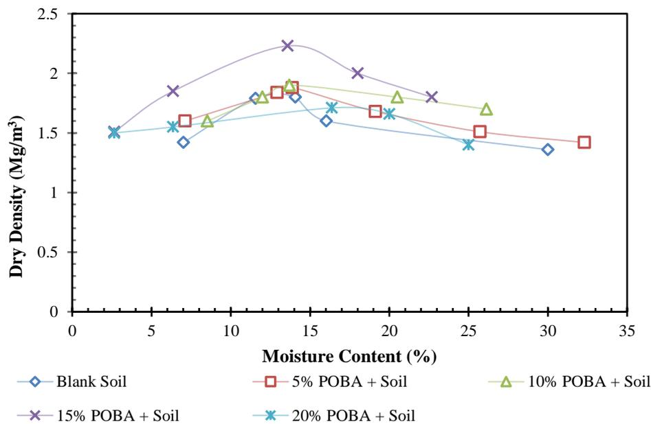
Fig. 10: Compaction Curve of Laterite soil with different percentages of geopolimer.
