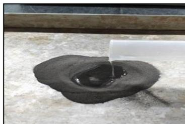
Fig 6: Alkaline solution mixed with POBA.
