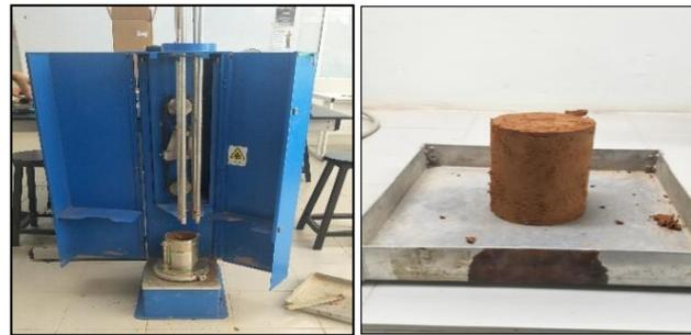
Fig. 9: Standard Proctor Machine and compaction sample.
