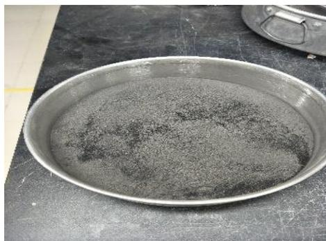
Fig. 4: Palm oil boiler ash passing 150  $\mu\text{m}$  sieve size.
