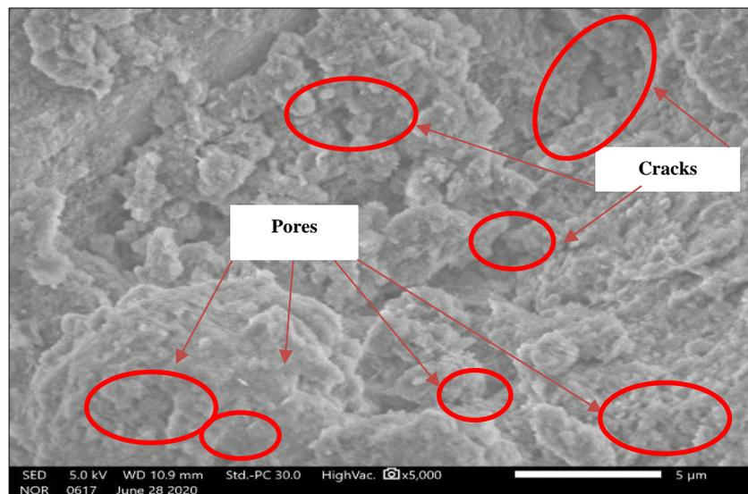
Fig. 13: SEM Samples of Plain Laterite (LS-P).
