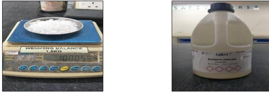
Fig. 5: (left) Sodium hydroxide in pellet form; (right) Sodium silicate in liquid form.
