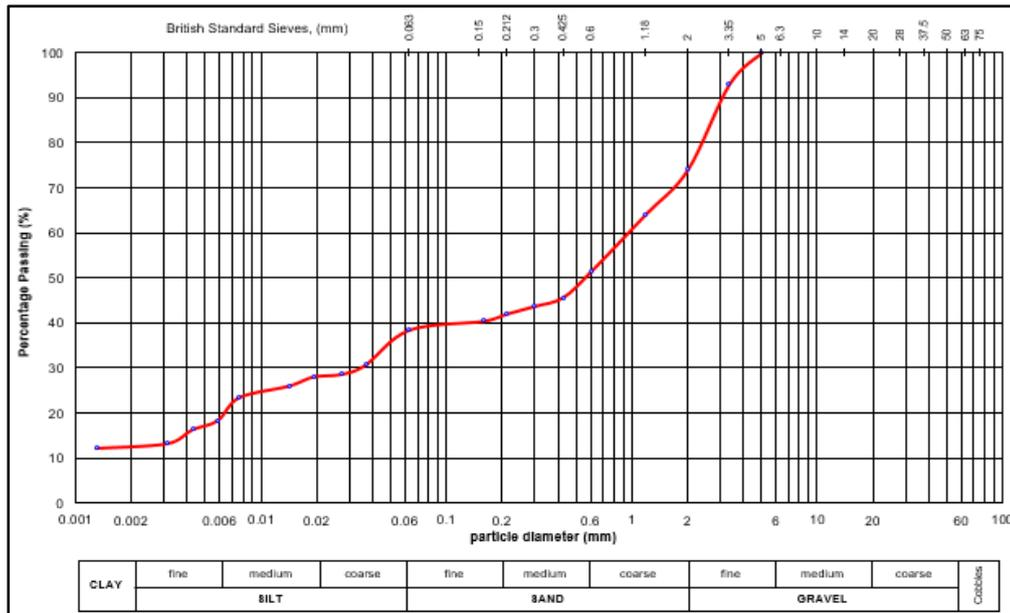
Fig. 2: Grain size distribution of laterite soil.
