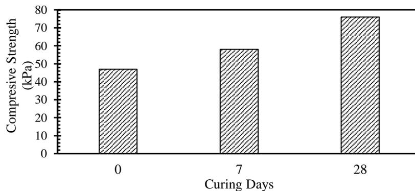
Fig. 12: The comparison of soil strength (LS-15.0 GPOBA) at zero, seven, and twenty-eight days of curing time.
