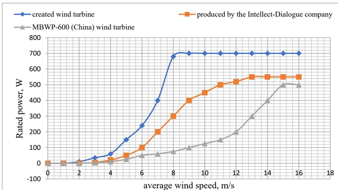
Fig. 11: Graph of the dependence of wind speed on the rated power of the developed wind power plant, as well as wind turbines produced in the Republic of Uzbekistan and a foreign prototype.
