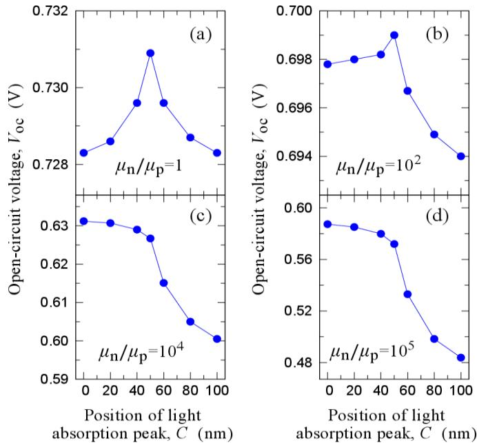
Fig. 4: Open-circuit voltage  $V_{oc}$  as a function of the position of the light absorption peak  $C$  when (a)  $\mu_n/\mu_p = 1$ , (b)  $\mu_n/\mu_p = 10^2$ , (c)  $\mu_n/\mu_p = 10^4$ , and (d)  $\mu_n/\mu_p = 10^5$ .
