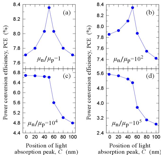
Fig. 7: Power conversion efficiency (PCE) as a function of the position of the light absorption peak  $C$  when (a)  $\mu_n/\mu_p = 1$ , (b)  $\mu_n/\mu_p = 10^2$ , (c)  $\mu_n/\mu_p = 10^4$ , and (d)  $\mu_n/\mu_p = 10^5$ .
