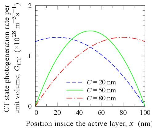
Fig. 2: Several profiles of the CT state photogeneration rate per unit volume  $G_{CT}$  that are used in this study. The expression for  $G_{CT}$  is given by Eq. (11).  $G_{CT}$  profile with light absorption peaks  $C$  at 0 nm, 40 nm, 60 nm and 100 nm are also used but are not shown in the figure.
