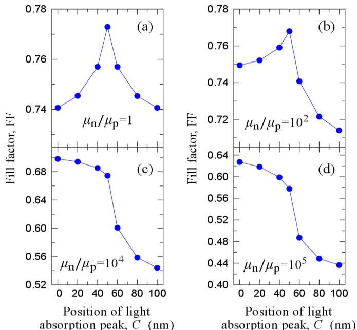
Fig. 6: Fill factor (FF) as a function of the position of the light absorption peak  $C$  when (a)  $\mu_n/\mu_p = 1$ , (b)  $\mu_n/\mu_p = 10^2$ , (c)  $\mu_n/\mu_p = 10^4$ , and (d)  $\mu_n/\mu_p = 10^5$ .
