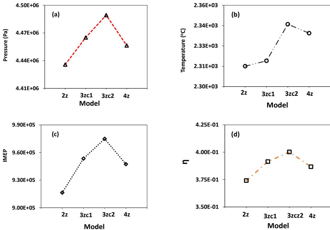
Fig. 4: Temperature, Indicated Mean Effective Pressure (IMEP) and thermal efficiency ( $\eta$ ) for 2-zone model (2z), 3-zone transitory model (3zc1), 3-zone segmented model (3zc2) and 4-zone model (4z) using 100% ethanol fuel.
