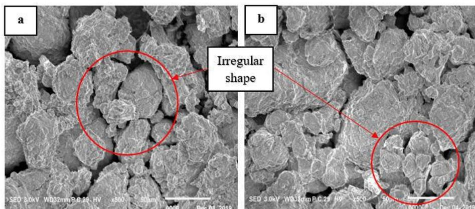
Fig.8. SEM micrographs of CaO-SiO<sub>2</sub> pellets ratio 80:20 before calcination at two different spots by magnification of 500X
