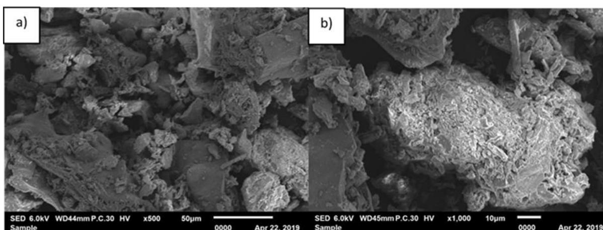
Fig 3: SEM micrographs of RHA at magnification of a) 500X and b) x1000X.
