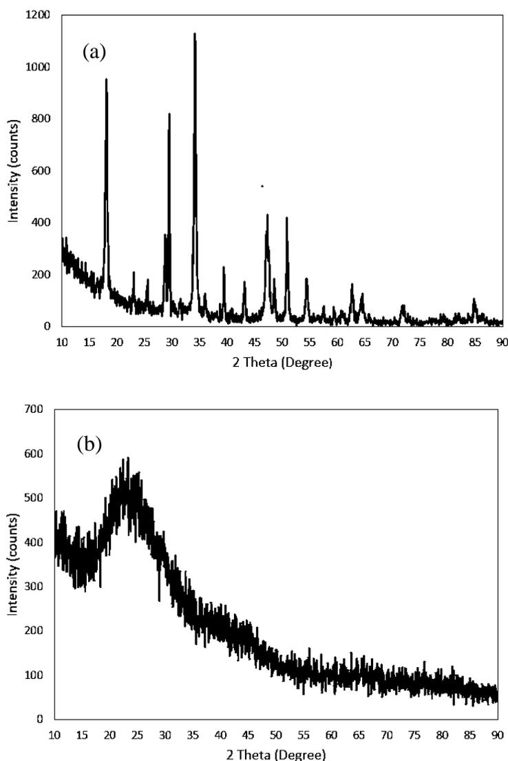
Fig.1. XRD pattern of a)  $\text{Ca}(\text{OH})_2$  and b) RHA.
