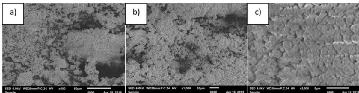
Fig. 2. SEM micrographs of  $\text{Ca}(\text{OH})_2$  at magnification of a) 500X, b) 1000X and c) 5000X.
