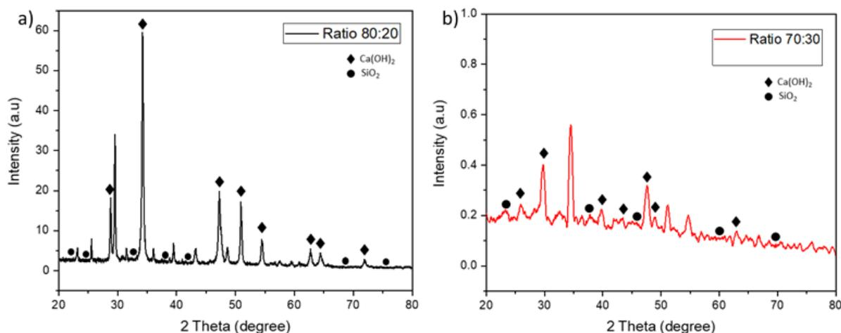
Fig. 6. XRD spectra for different ratio of CaO-SiO<sub>2</sub> before calcination, (a) 80: 20 and (b) 70:30
