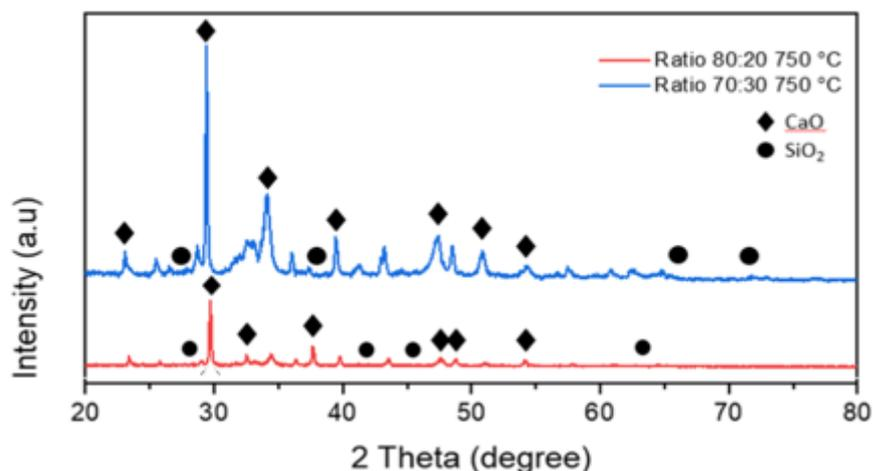
Fig.9. XRD spectra for different ratio of CaO-SiO<sub>2</sub> pellet calcined at 750°C
