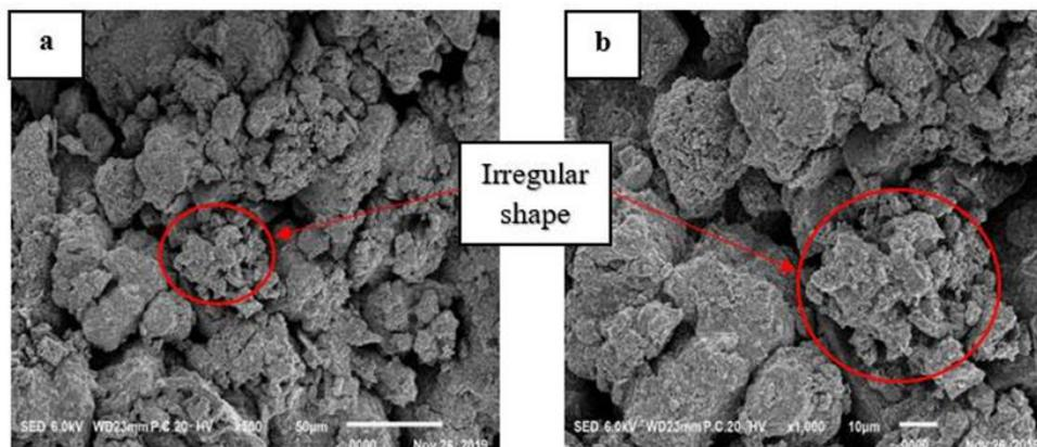
Fig.7. SEM micrographs of CaO-SiO<sub>2</sub> pellets ratio 70:30 before calcination at different magnification a) 500X and b) 1000X
