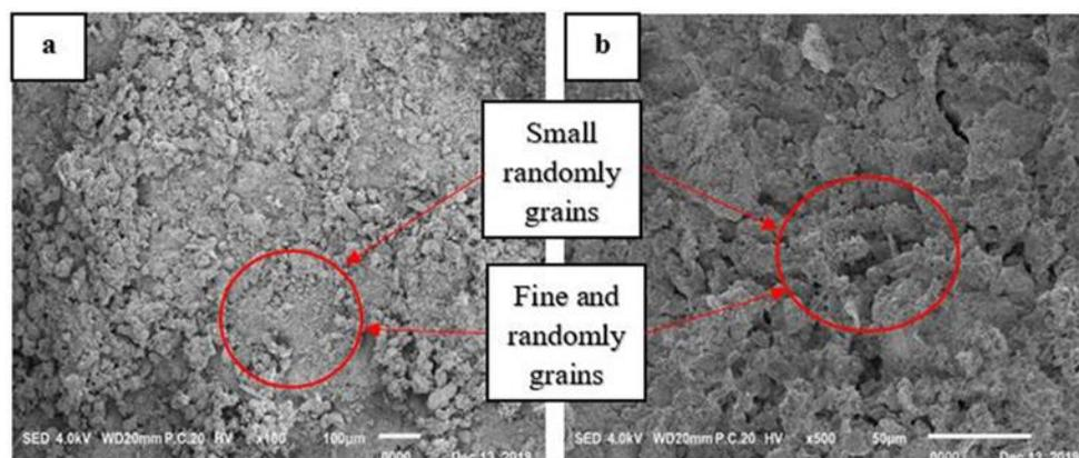
Fig.11. SEM micrographs of CaO-SiO<sub>2</sub> pellets ratio 70:30 after calcination at 750 °C with different magnification a) 100X and b) 500X.
