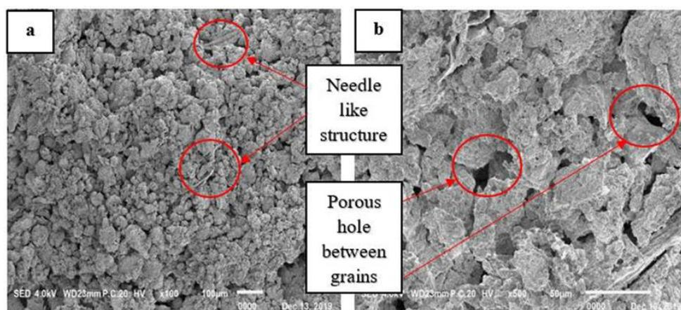
Fig.10. SEM micrographs of CaO-SiO<sub>2</sub> pellets ratio 80:20 after calcination at 750°C with different magnification a) 100X and b) 500X.
