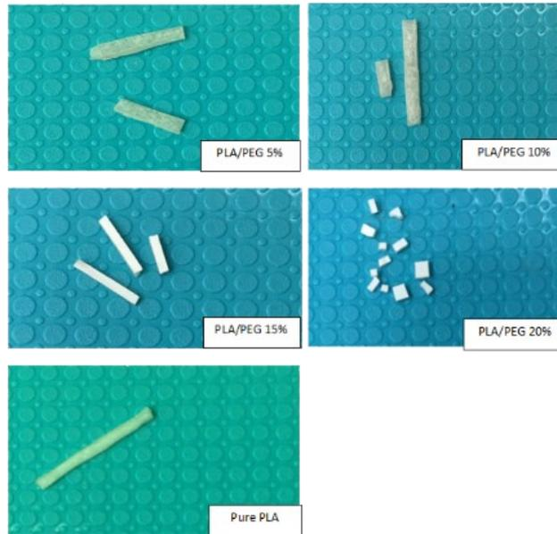
Fig. 5: Micrograph of samples after 34th week of degradation test.
