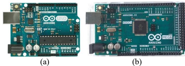
Fig. 4: CDUs: (a) Arduino Uno, (b) Arduino MEGA.
