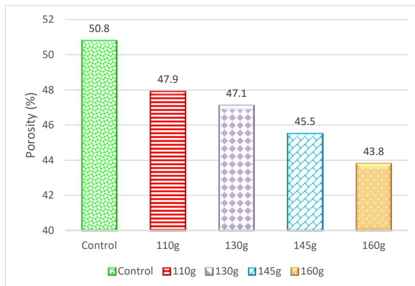
Fig. 5: Porosity of LFC specimens confined with different weights per area ( $\text{g/m}^2$ ) of fibremesh at day-28.
