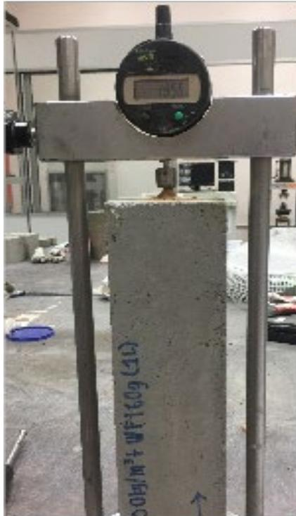
Fig. 4: Setup for drying shrinkage test.
