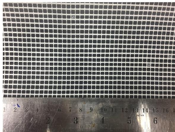
Fig. 1: Physical features of the fibremesh.
