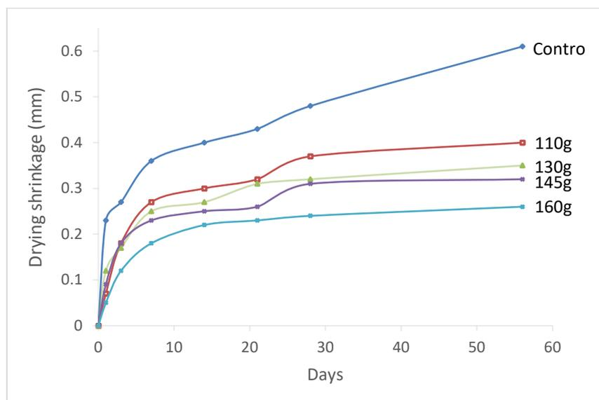
Fig. 7: Drying shrinkage of LFC specimens confined with different weight per area (g/m<sup>2</sup>) of fibremesh.
