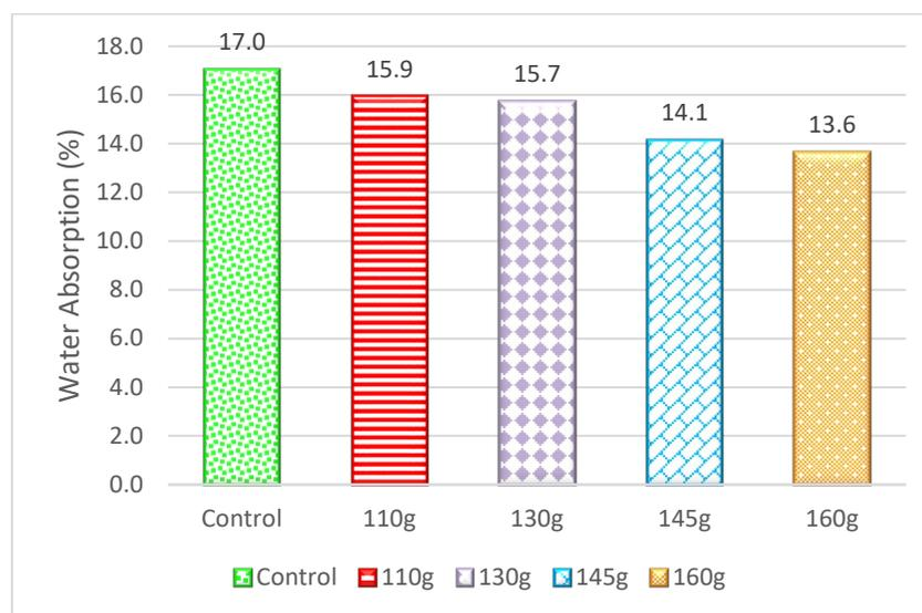
Fig. 6: Water absorption capacity of LFC specimens confined with different weights per area (g/m<sup>2</sup>) of fibremesh at day-28.
