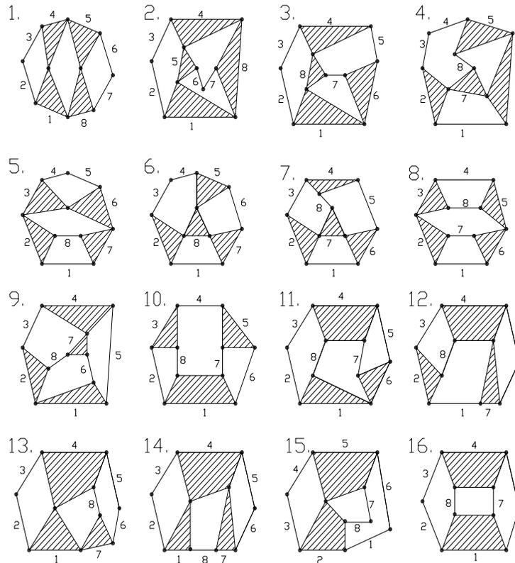
Fig. 3: Eight link single degree of freedom non-isomorphic planar kinematic chains.
