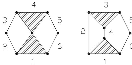
Fig. 1: Watt’s and Stephenson’s six link kinematic chain.
