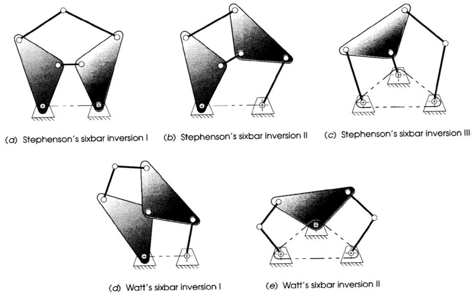
Fig. 2: Inversion's of Watt's and Stephenson's kinematic chain.
