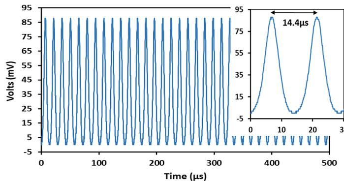
Fig. 3: The measured oscilloscope trace for the Q-switched laser at 69.97 kHz. The inset shows the free spectral range for successive pulses.
