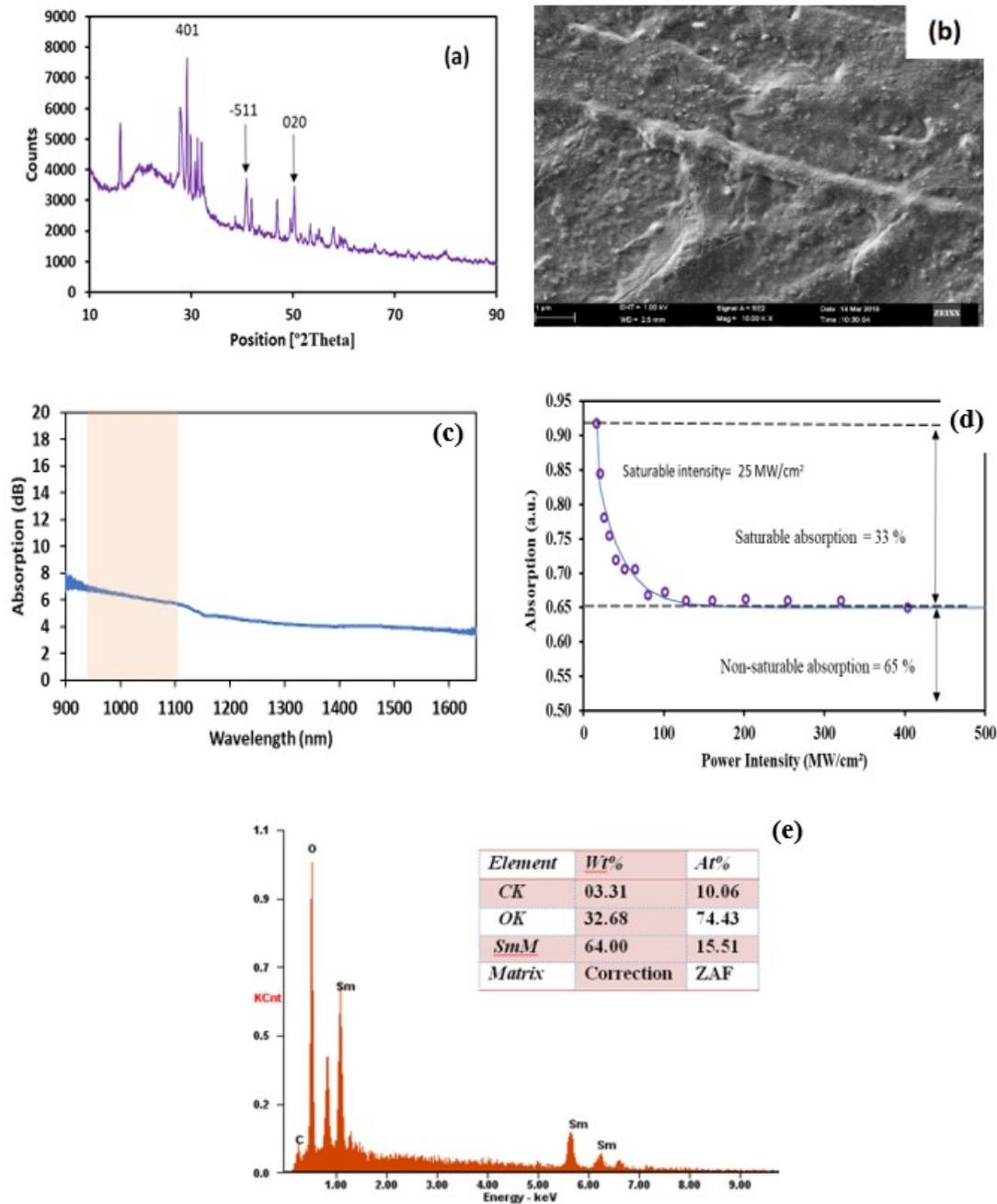
Fig. 1: Characterization of  $\text{Sm}_2\text{O}_3$  PVA film as SA (a) XRD (b) FESEM (c) Linear absorption profile (d) Nonlinear absorption profile (e) Energy dispersive X-ray.
