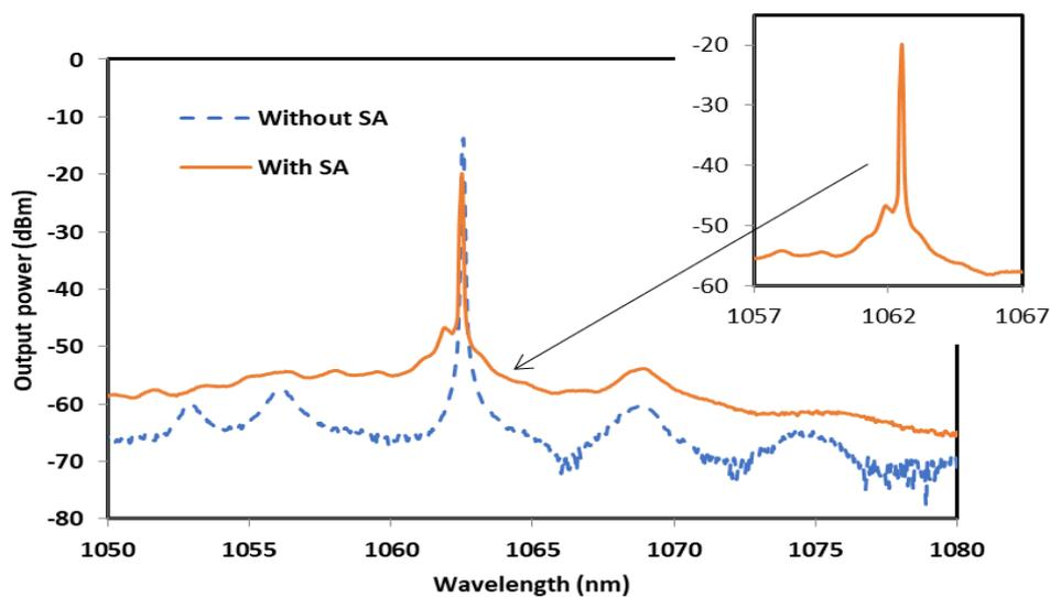
Fig. 5: Spectrum of CW laser (without SA) and Q-switched laser (with SA).
