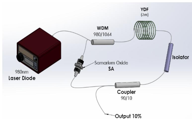
Fig. 2: The schematic for the Q-switched ytterbium laser setup incorporating  $\text{Sm}_2\text{O}_3$  based saturable absorber (SA).
