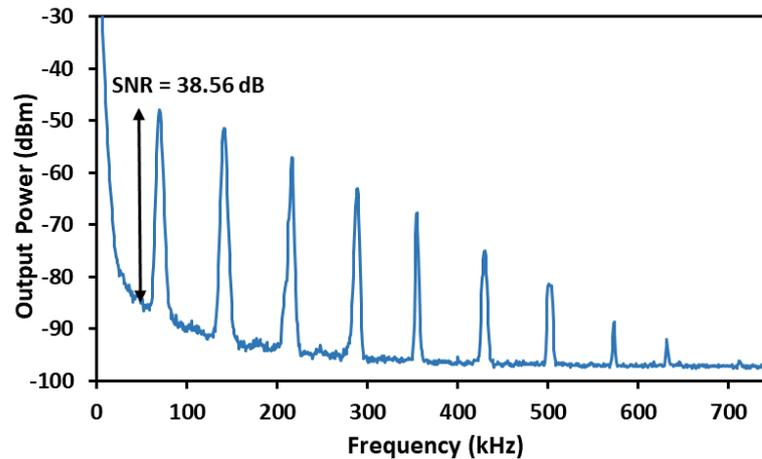
Fig. 6: Q-switched YDFL RF spectrum when the pump power is 57 mW.
