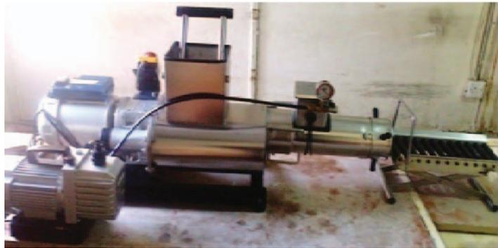
Fig. 4: Clay extrusion device.
