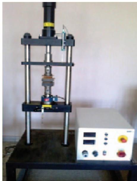
Fig. 8: Sample under compressive strength test.
