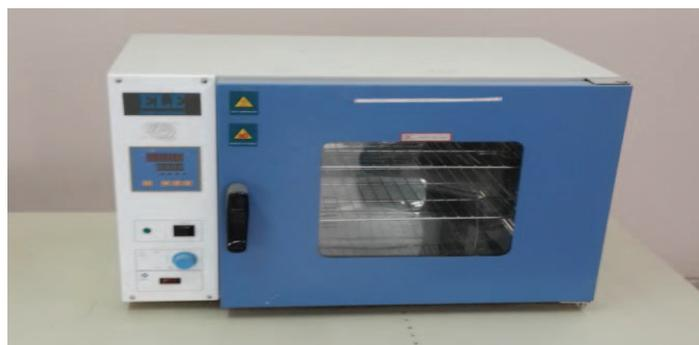
Fig. 5: Curing and drying furnace.
