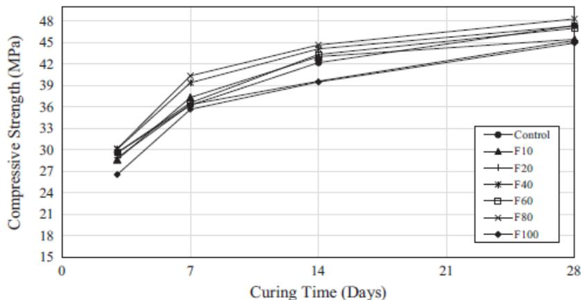
Fig. 2: Concrete strength performance with POC as replacement of fine aggregates [8].
