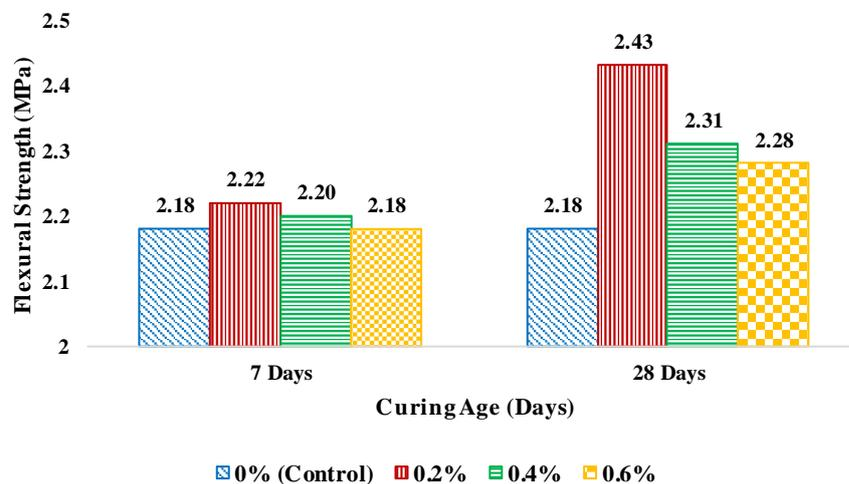
Fig. 10: Concrete flexural strength at curing periods of 7 and 28 days.
