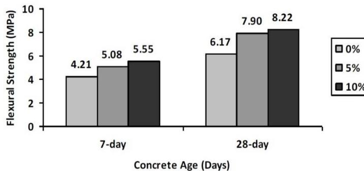
Fig. 3: Flexural strength result of POC concrete and conventional concrete [9].
