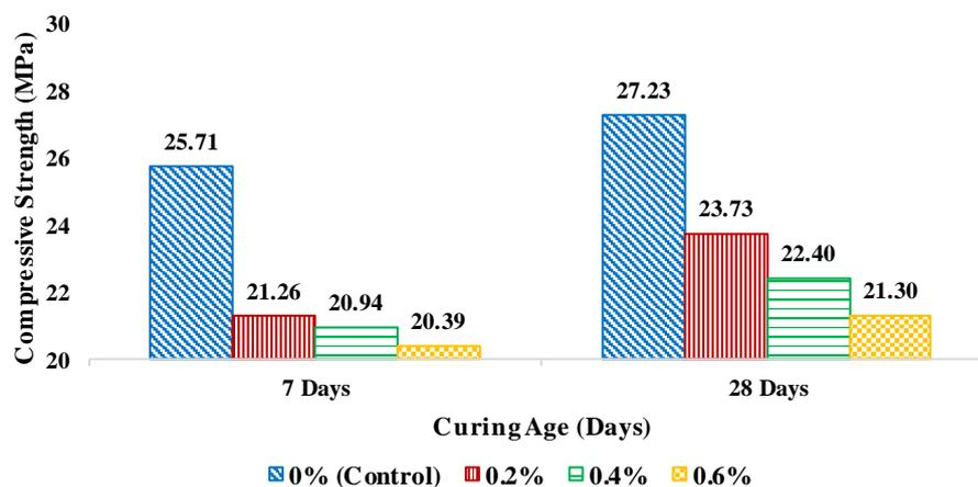
Fig. 9: Compressive strength of fiber reinforced concrete at different curing periods
