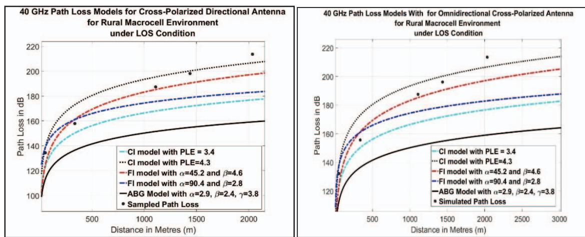
Fig. 3: 40 GHz rural macrocell simulated path loss model alongside scatter plot under LOS condition.
