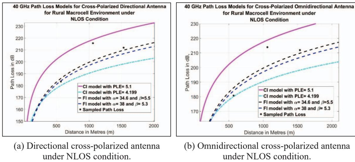
Fig. 4: 40 GHz rural macrocell simulated path loss model under NLOS condition.
