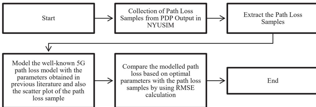
Fig. 2: Research flow for finding the accurate path loss model for 5G networks in rural macrocell environment in Malaysia.
