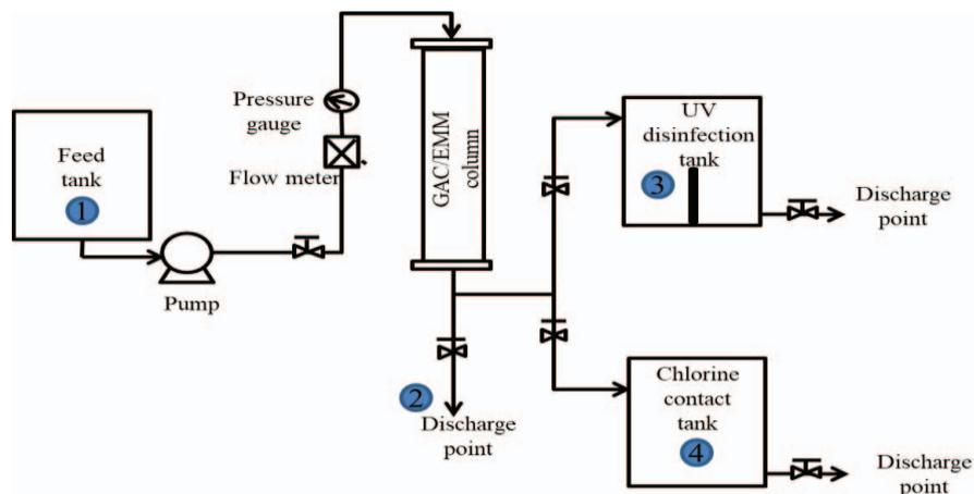
Fig. 2: Schematic diagram of bench-scale integrated disinfection system (GAC/EMM column-chlorination and GAC/EMM column-UV) with sampling points: (1) at feed tank (2) at discharge point of GAC/EMM column (3) at UV disinfection tank (4) at chlorine contact basin.
