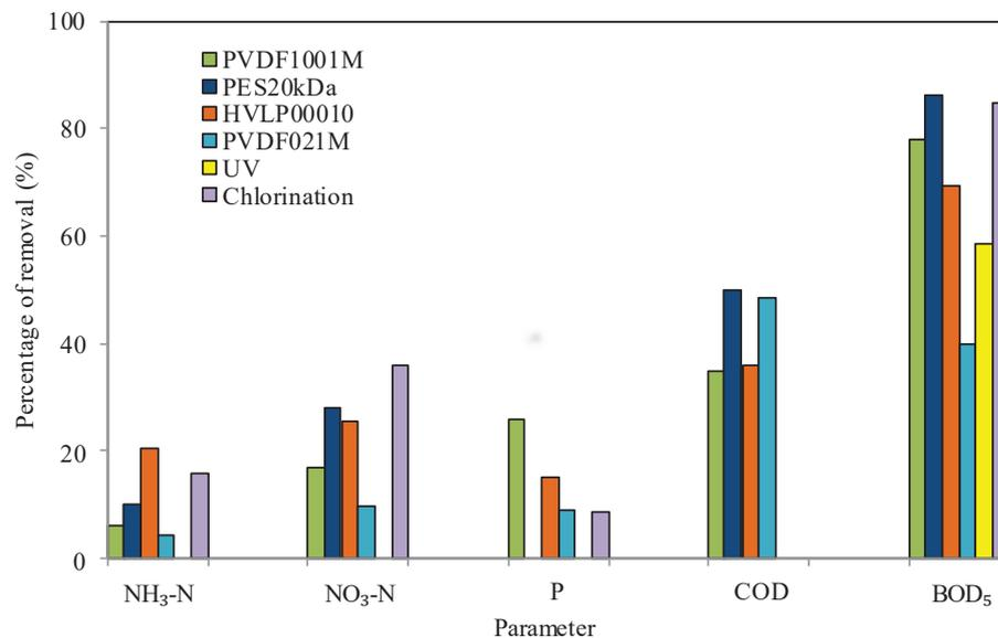
Fig. 5: Performance of single disinfection unit.
