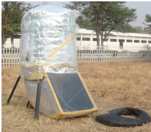
Fig. 3: Fabricated solar biogas digester with flexible gas-holder.
