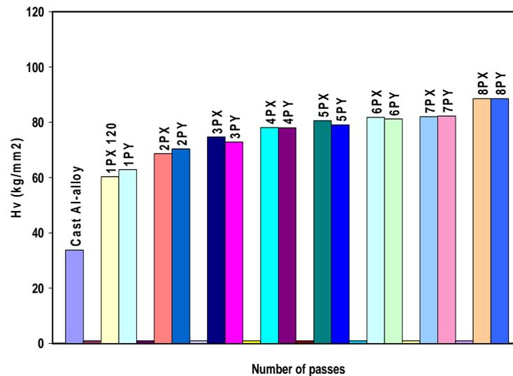
Fig. 5: The average values of Vickers microhardness (Hv) for the cast and ECAPed Al-Si workpieces on the X and Y planes, showing alongside the number of passes through the die with  $\Phi=120^{\circ}$  and  $\Psi=0^{\circ}$ . (P: Pass, X: X-plane and Y: Y-plane).
