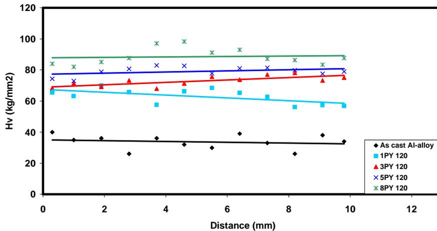
Fig. 8: Vickers microhardness at Y-plane for cast Al-Si alloy, 1, 3, 5 and 8 passes through the die with  $\Phi=120^0$  and  $\Psi=0^0$  from the bottom (near to  $\Psi$ ) to the top (near to  $\Phi$ ) of the Workpiece.
