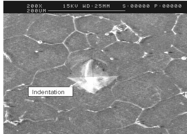
Fig. 3: SEM photomicrograph showing microstructures of the Al-Si alloy as cast (x 200 marker  $200\ \mu\text{m}$ ).
