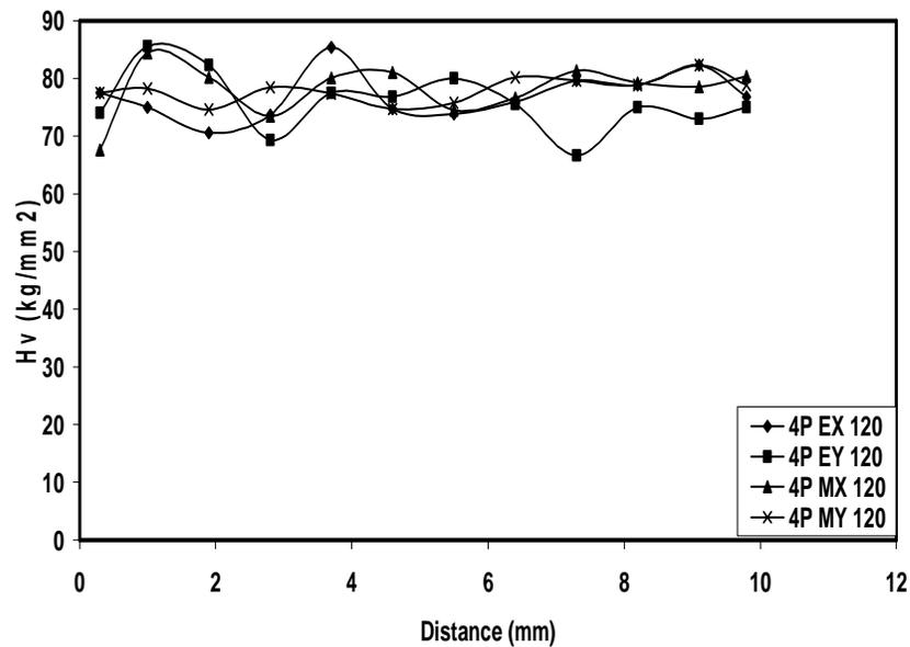
Fig. 9: Vickers microhardness from the bottom to the top of the Al-Si workpiece at two locations for 4 passes through the die with  $\Phi=120^0$  and  $\Psi=0^0$  on the X and Y planes. (E: end of the workpiece that is in touch with the Plunger); (M: middle of the workpiece); (X: X-plane and Y: Y-plane); (P: pass).
