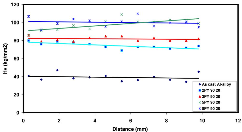
Fig.11: Shows the Vickers microhardness (Hv) profiles at Y-plane along transverse distance from the bottom (near to  $\Psi$ ) to the top (near to  $\Phi$ ) of the cast, 2, 3, 5 and 8 ECAPed Al-Si alloy workpieces through the die with  $\Phi=90^0$  and  $\Psi=20^0$ .
