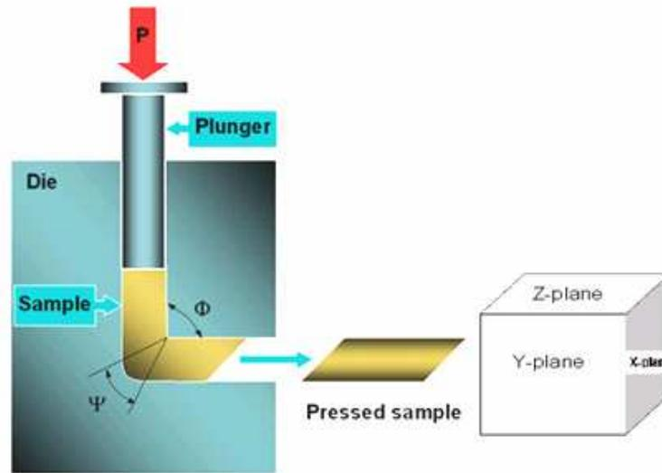
Fig. 1: Angles for equal channel angular pressing and ECAPed workpiece.
