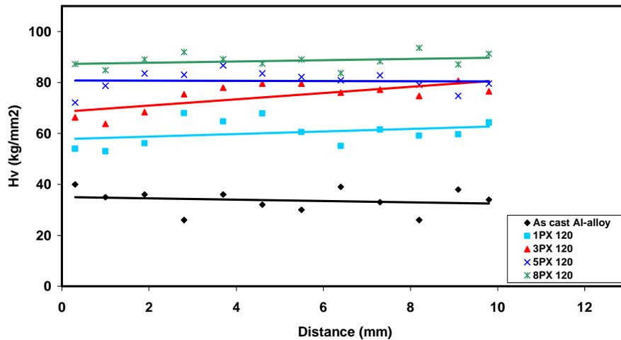
Fig. 7: Vickers microhardness at X-plane for cast Al-Si alloy, 1, 3, 5 and 8 passes through the die with  $\Phi=120^0$  and  $\Psi=0^0$  from the bottom (near to  $\Psi$ ) to the top (near to  $\Phi$ ) of the Workpiece.
