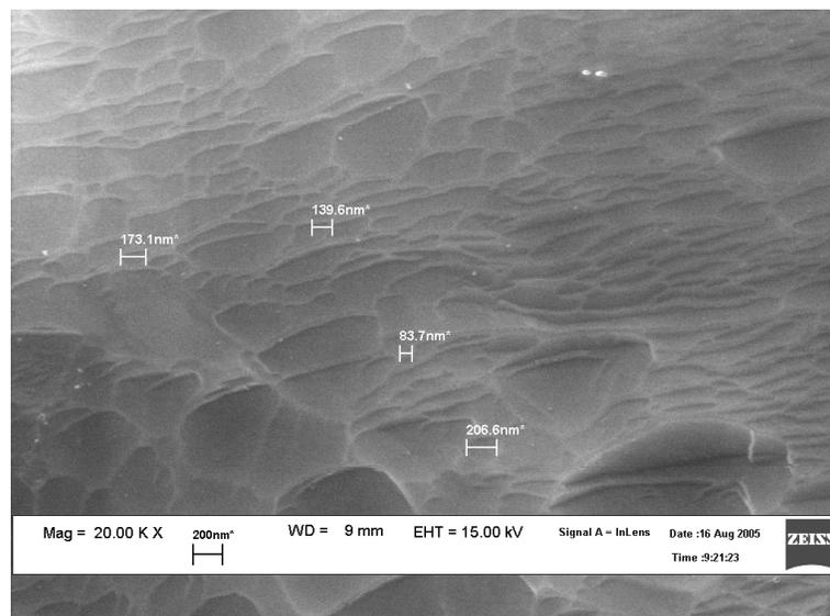
Fig. 6: SEM photomicrograph showing microstructures of the Al-Si alloy pressed through the die with  $\Phi=120^{\circ}$  and  $\Psi=0^{\circ}$  using route B<sub>C</sub>; after 2 passes on the X-plane.
