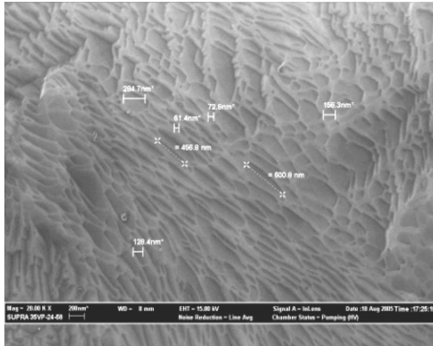
Fig.12: Microstructure of ECA pressed Al-Si alloy after 7 passes through the die with  $\Phi=90^0$  and  $\Psi=20^0$ , using route B<sub>C</sub>.
