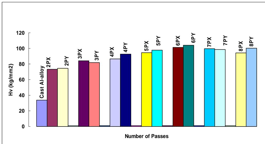
Fig. 13: The average values of Vickers microhardness (Hv) for the cast and ECAPed Al-Si workpieces at the X and Y-planes shown alongside the number of passes through the die with  $\Phi=90^0$  and  $\Psi=20^0$ . (P: pass, X: X-plane and Y: Y-plane).
