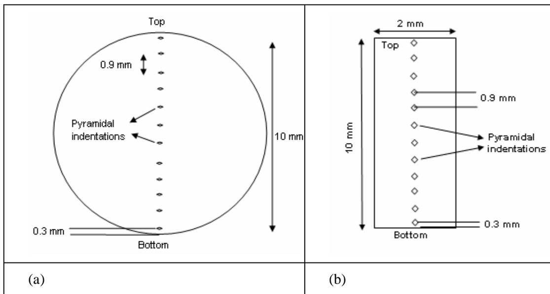
Fig. 2: Sketch of pyramidal Vickers indentations on (a) X-plane, (b) Y-plane.
