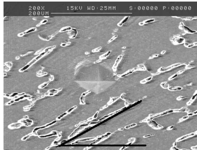
Fig. 4: SEM photomicrograph showing microstructures of the Al-Si alloy after 1 pass on the Y-plane using a die with  $\Phi=120^\circ$  and  $\Psi=0^\circ$  using route B<sub>C</sub>.
