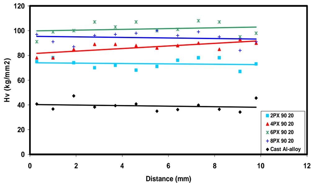
Fig.10: Vickers microhardness (Hv) profiles at X-plane along the transverse distance from the bottom (near to  $\Psi$ ) to the top (near to  $\Phi$ ) of the cast, 2, 4, 6 and 8 ECAPed Al-Si alloy workpieces through the die with  $\Phi=90^0$  and  $\Psi=20^0$ .
