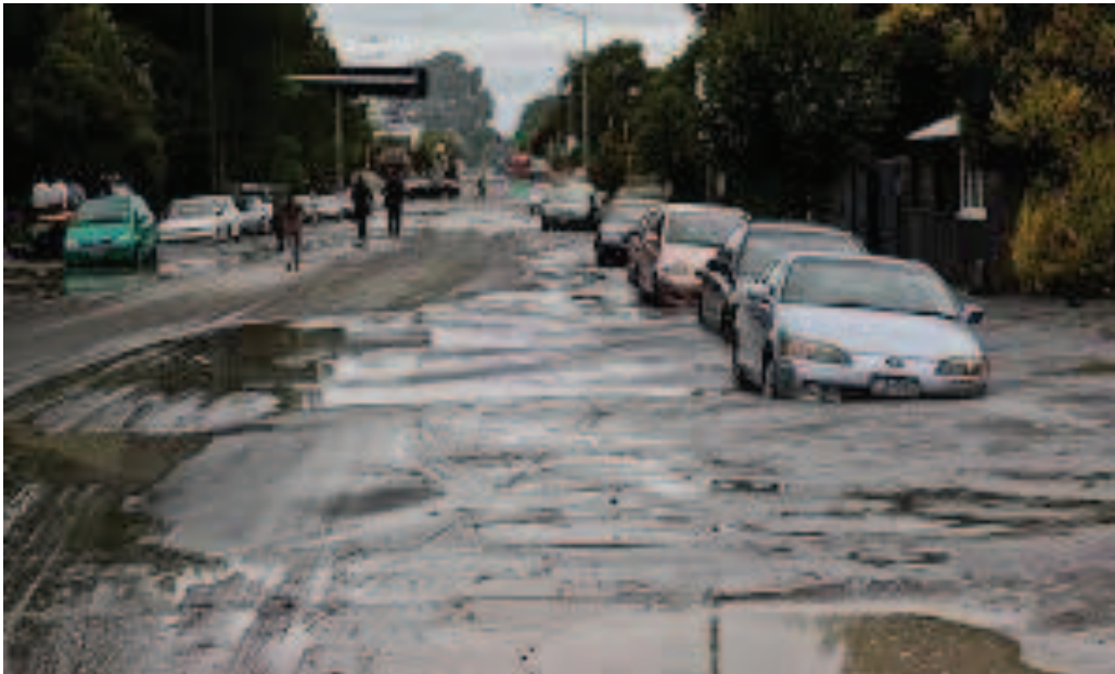
Fig. 1: The impact of liquefaction in Christchurch, New Zealand [6].
