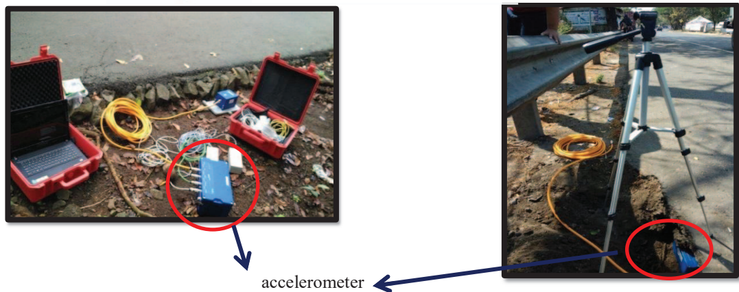
Fig. 5: Installation of the accelerometer in the field.
