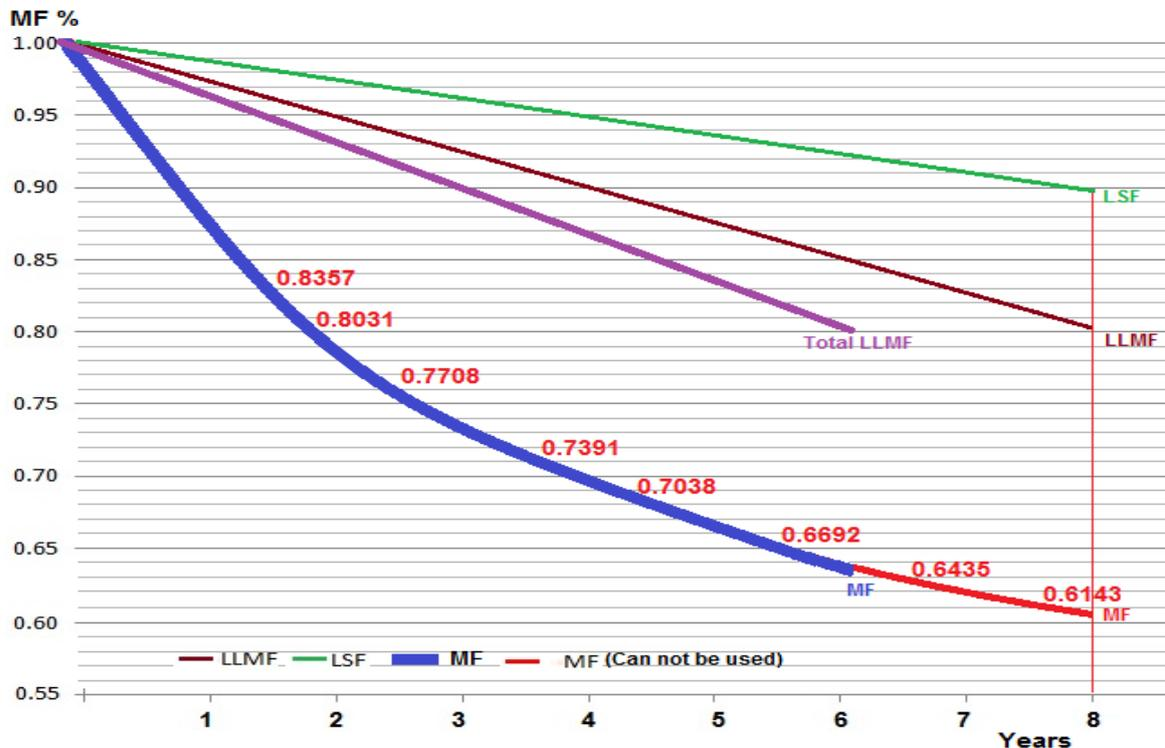
Fig. 7. Optic performance change depending on operating for LED luminaires
