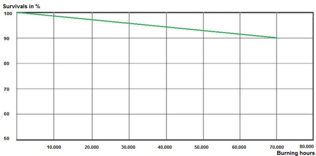
Fig. 6. Line of LSF for LED lamps.
