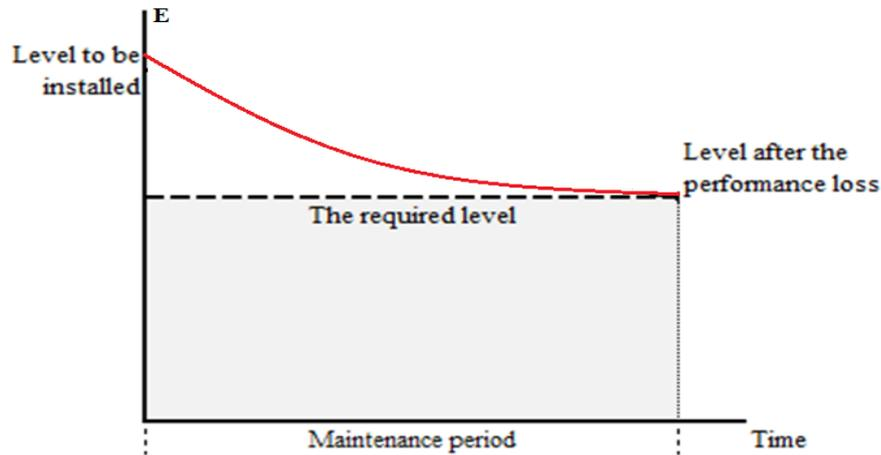
Fig. 1. Tolerance range associated with Maintenance Factor as regards performance loss [5].
