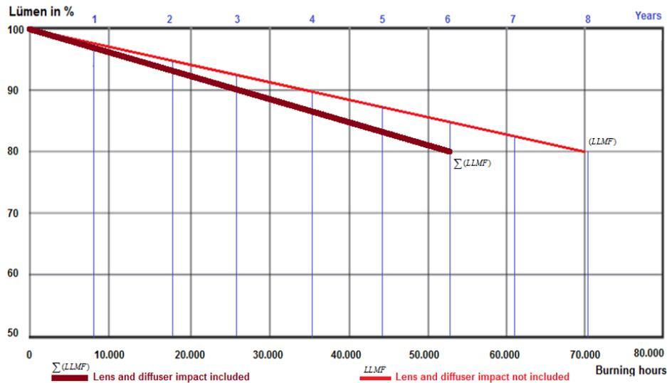
Fig. 5. Decrease in Luminous Flux depending on the operating time of LED lamps.
