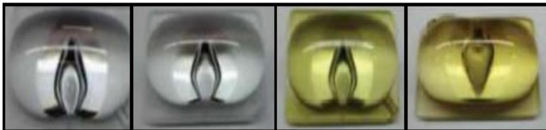
Fig. 4. Optical variance caused by use of LED lens at UV/65°C for 6000 hours.
