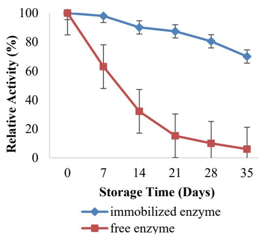
Fig. 7: Storage stability test of immobilized and free lipase.
