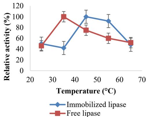
Fig. 2: Optimum temperatures for both immobilized and free lipase.
