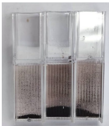
Fig. 3. The different ratios tested in synthesizing magnetic silver nanoparticles. 1:9 (left), 1:2 (middle), 1:3 (right).
