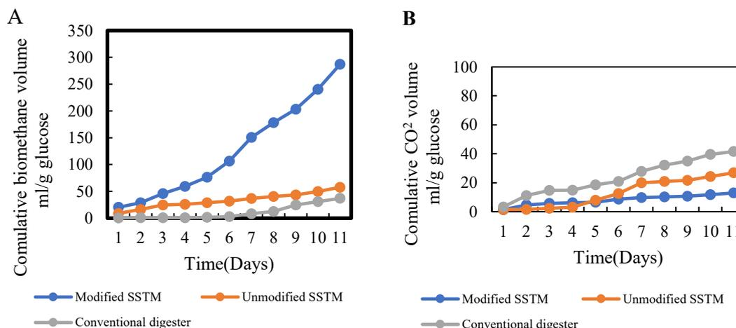
Fig. 7. Cumulative biomethane(A) and  $\text{CO}_2$  production(B) of conventional digester, Modified system, and unmodified system.
