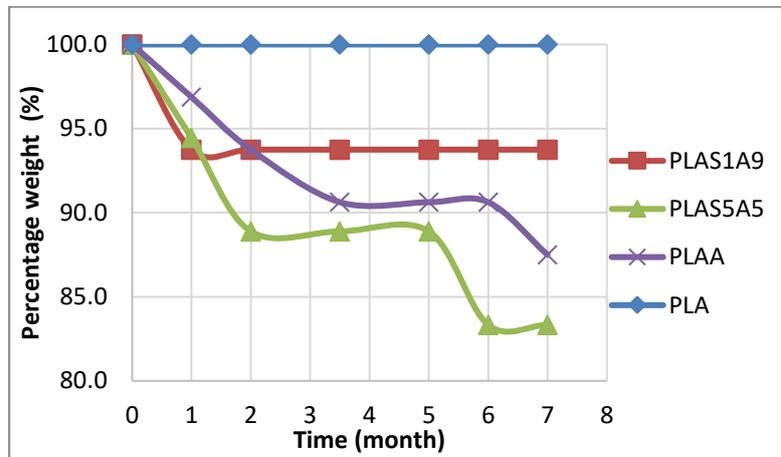
Fig. 2. Percentage weight of PLA and PLA composites by microbial degradation
