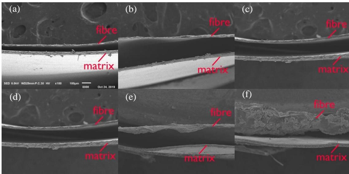
Fig. 3. SEM micrograph of cross section of (a)PLAS1A9 (b)PLAS5A5 and (c)PLAA before the degradation. Cross section off (d)PLAS1A9 (e)PLAS5A5 and (f)PLAA after the degradation.
