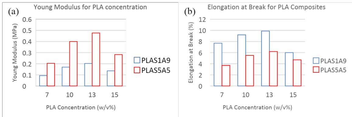
Fig. 1. The comparison of PLA composites in (a) Young's Modulus and (b) Elongation at break.
