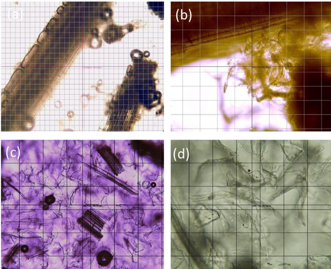
Figure 4: Optical microscope image of sugarcane bagasse with (a) 100× and (b) 400× magnifications before pretreatment (control) and (c) 100× and (d) 400× magnifications after SSF.
