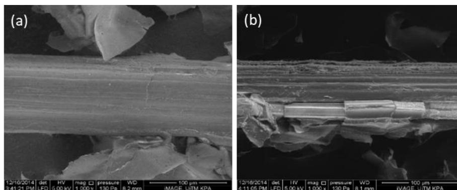
Figure 5: FESEM micrographs at 1000× magnification of (a) crude sugarcane bagasse and (b) sugarcane bagasse after SSF.
