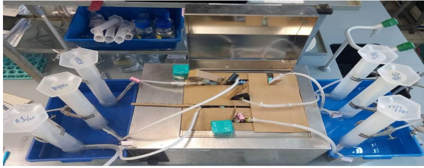
Fig. 2. Experimental anaerobic digestion setup maintained at 37 °C.
