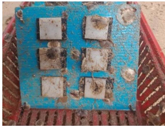
Fig. 8. Biofouling adherence to the high-density polyethylene (HDPE) pipe coupons
