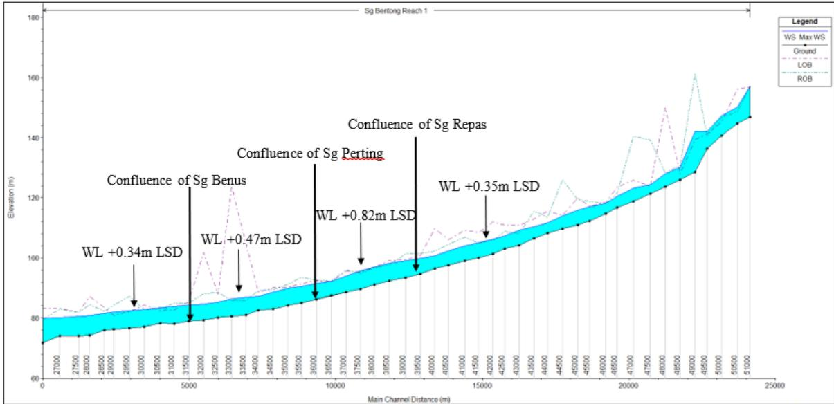
Fig. 14. Max Water Level Profile of Sg Bentong (HEC-RAS): 6 Hours 100-Years ARI (Option 5-Rainwater Harvesting System)
