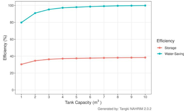
Fig. 6. Water-saving and storage efficiency vs proposed tank size
