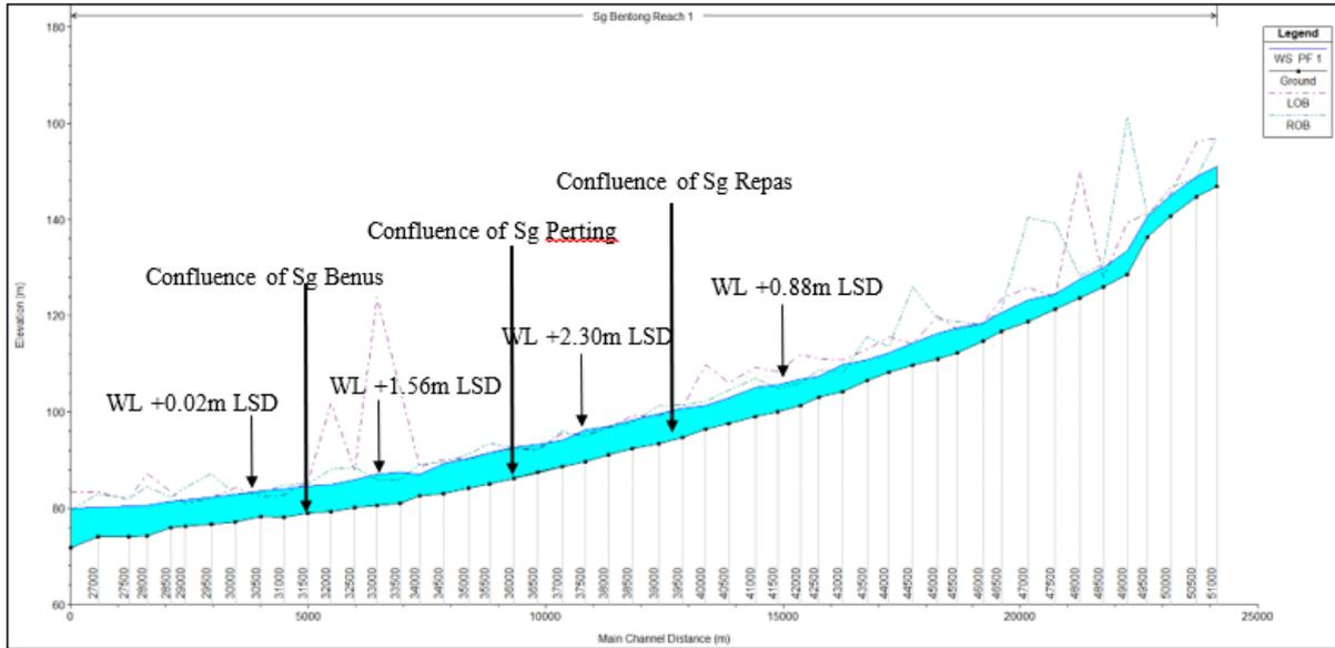
Fig. 10. Max Water Level Profile of Sg Bentong (HEC-RAS): 6 Hours 100-Years ARI (Option 5-Proper Land Use Allocation/Planning)
