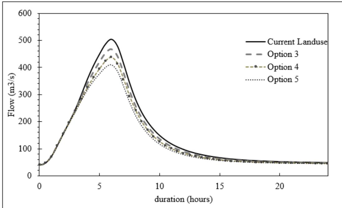
Fig. 8. Simulated Flow Hydrographs of Sg Bentong 100-year ARI 6 Hours Design Rainfall- Proper Land Use Allocation
