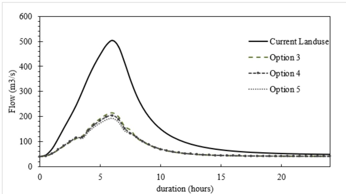
Fig. 17. Simulated Flow Hydrographs of Sg Bentong 100-Years ARI 6 Hours Design Rainfall- Integrated Non-Structural Flood Mitigations
