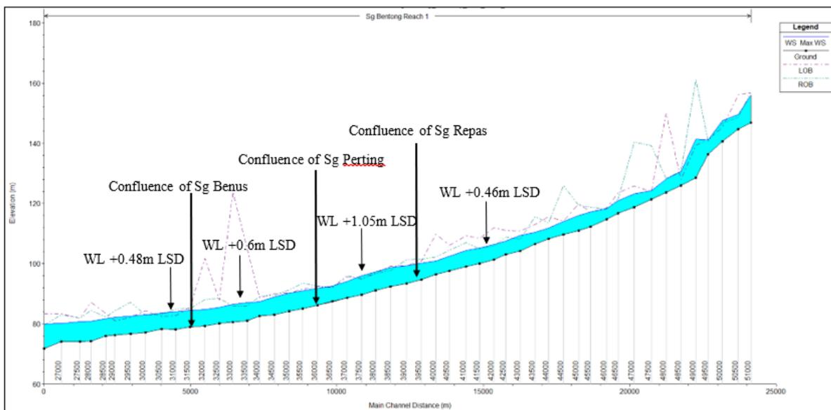
Fig. 13. Max Water Level Profile of Sg Bentong (HEC-RAS): 6 Hours 100-Years ARI (Option 3-Rainwater Harvesting System)
