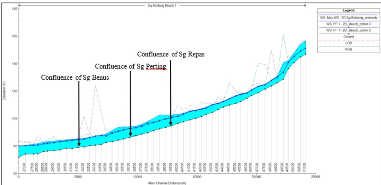
Fig. 11. Comparison of Max Water Level Profile of Sg Bentong (HEC-RAS): 6 Hours 100-Years ARI- Proper Land Use Allocation/Planning
