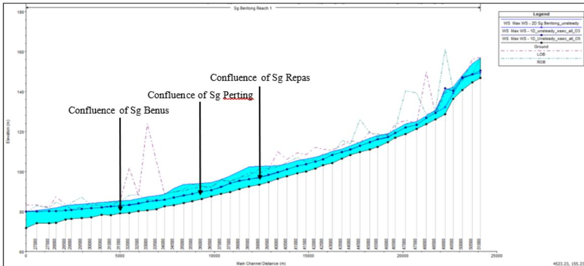
Fig. 20. Comparison of Max Water Level Profile of Sg Bentong (HEC-RAS): 6 Hours 100-Years ARI- Integrated Non-Structural Flood Mitigations
