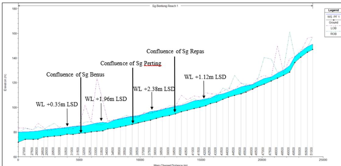
Fig. 9. Max Water Level Profile of Sg Bentong (HEC-RAS): 6 Hours 100-years ARI (Option 3-Proper Land Use Allocation/Planning)
