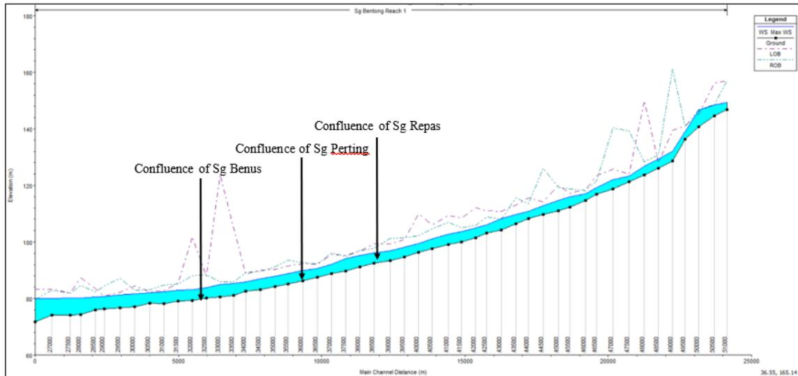
Fig. 18. Max Water Level Profile of Sg Bentong (HEC-RAS): 6 Hours 100-Years ARI (Option 3- Integrated Non-Structural Flood Mitigations)
