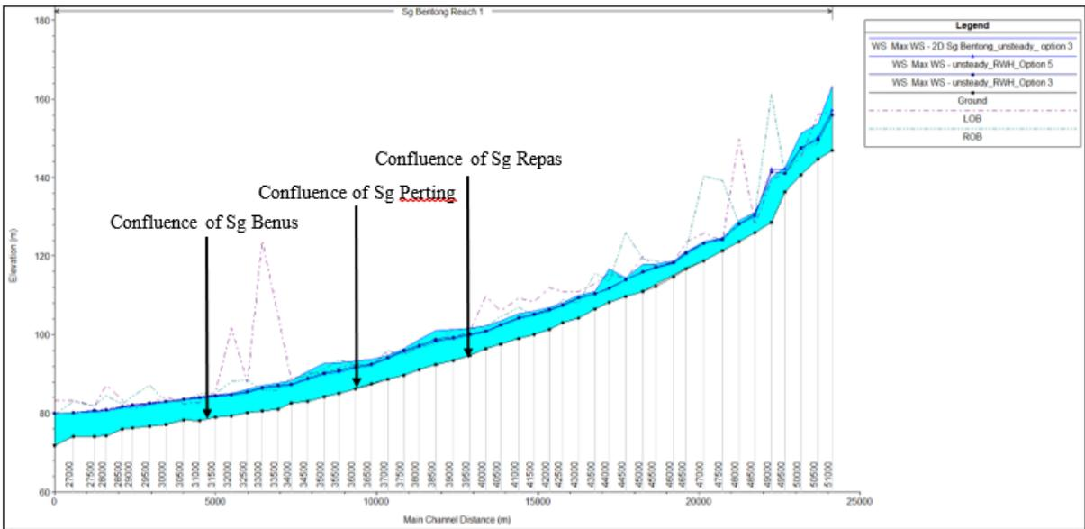
Fig. 15. Comparison of Max Water Level Profile of Sg Bentong (HEC-RAS): 6 Hours 100-Years ARI- Rainwater Harvesting System
