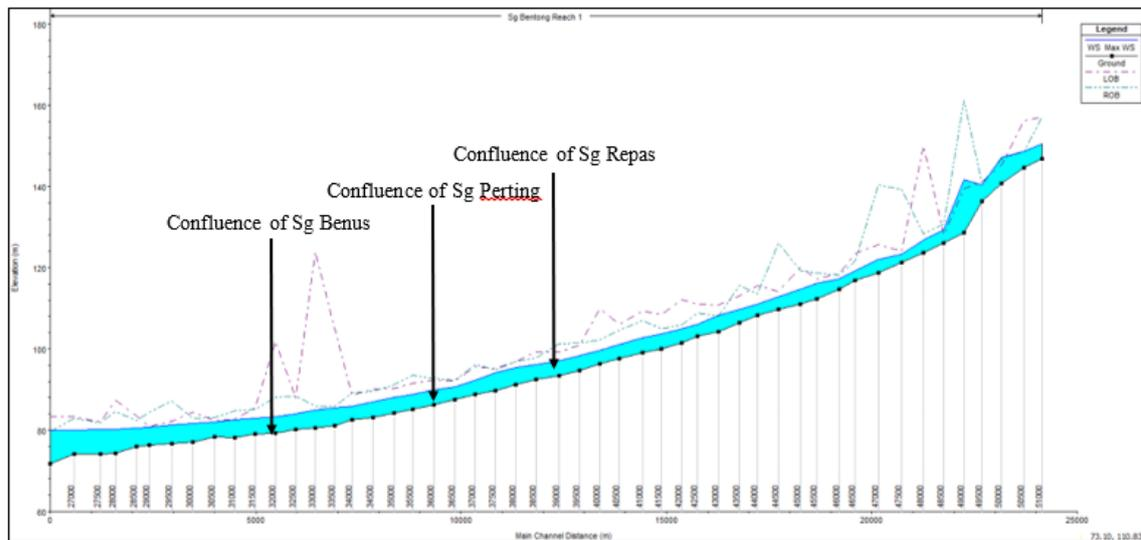
Fig. 19. Max Water Level Profile of Sg Bentong (HEC-RAS): 6 Hours 100-Years ARI (Option 5- Integrated Non-Structural Flood Mitigations)
