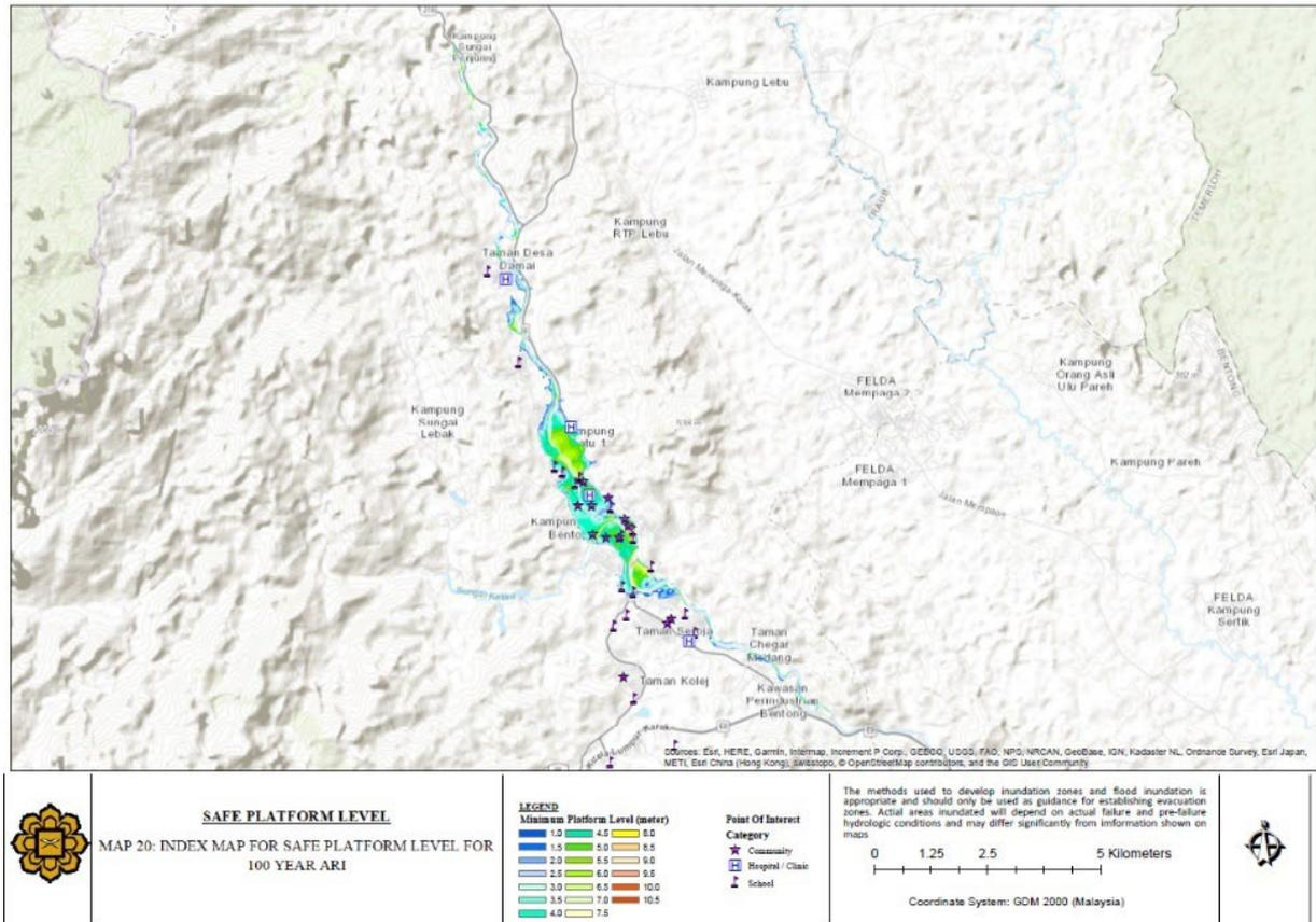
Fig. 25. Index map for safe platform level for 100 years ARI.
