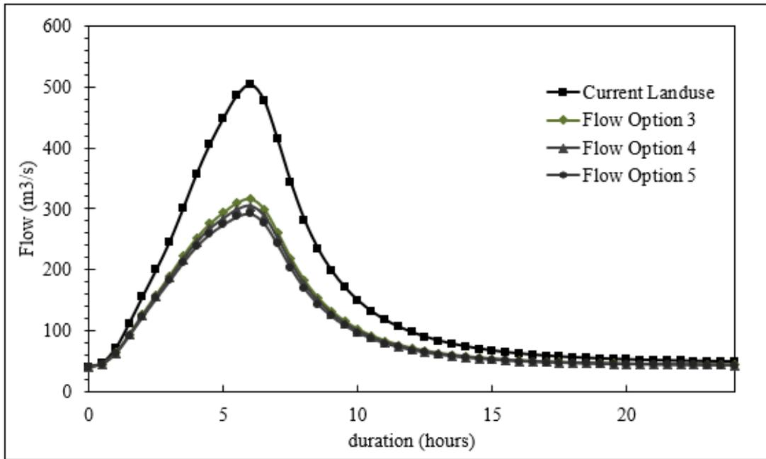
Fig.12. Simulated Flow Hydrographs of Sg Bentong 100-Years ARI 6 Hours Design Rainfall- RWHS
