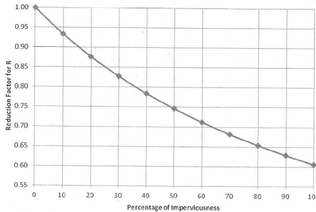
Fig. 3. Reduction Factor for R in Relationship with Imperviousness.
