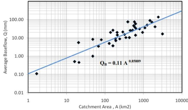
Fig. 2. Relationship of Baseflow and Catchment Area (HP No. 27(2010)).
