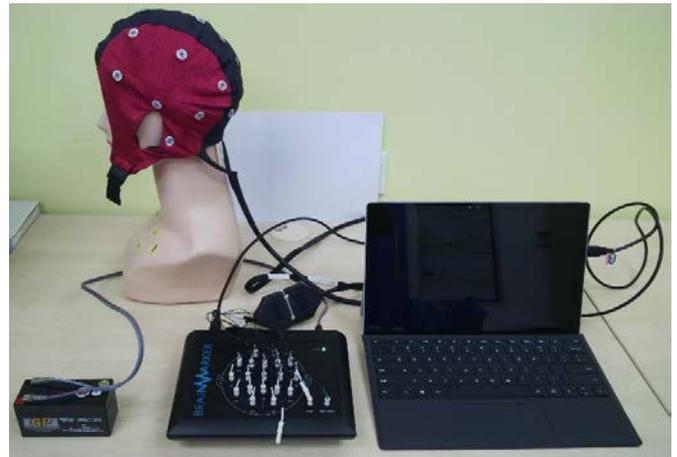
Figure 1. EXG Brain Marker Mobile EEG Device
