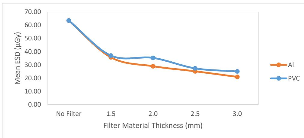
**Figure 1.** Graph shows means entrance surface dose (ESD) values versus increment in filter material thickness
