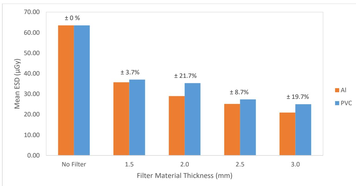
**Figure 2.** Graph shows the percentage difference between Al and PVC filter with the equal thickness
