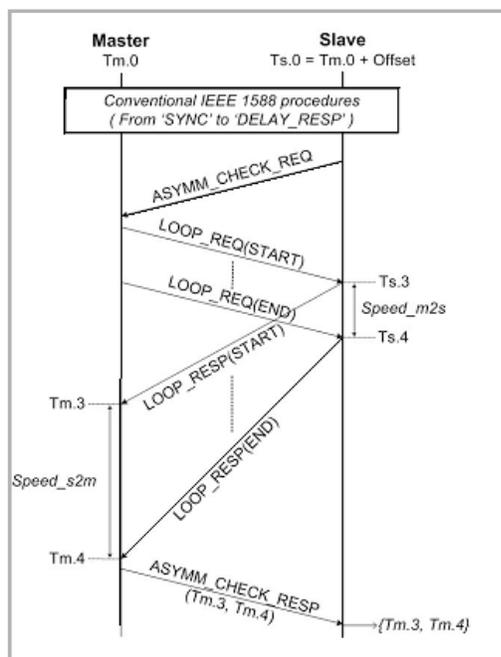
Fig. 3: Block burst transmission for the asymmetric ratio calculation [3]
