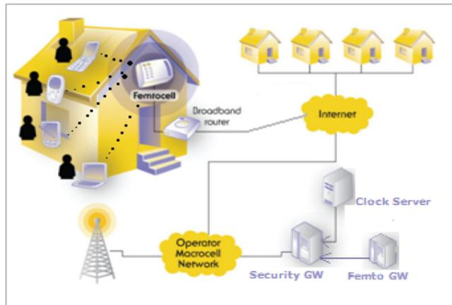
Fig. 1: A femtocell network architecture [2]
