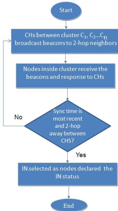
Fig. 8: Proposed Intermediate Node (IN) selection procedure.
