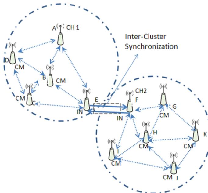
Fig. 9: Proposed Inter-cluster synchronization procedure.
