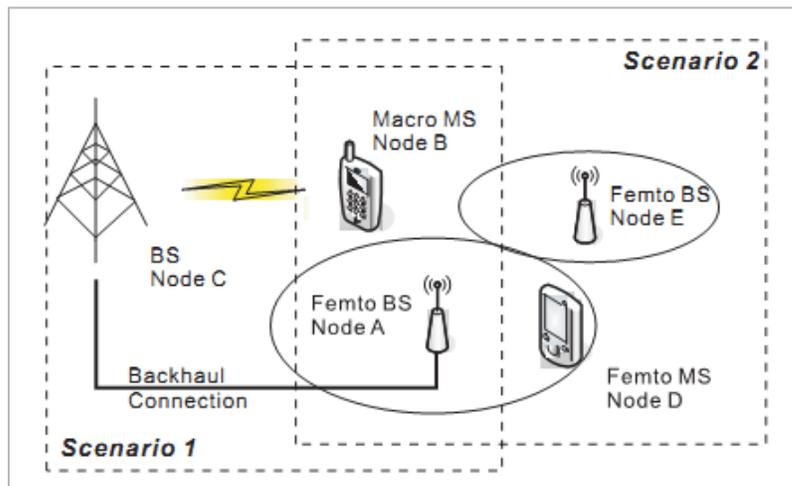
Fig. 4: The Two Femtocell Synchronization Scenarios [8].
