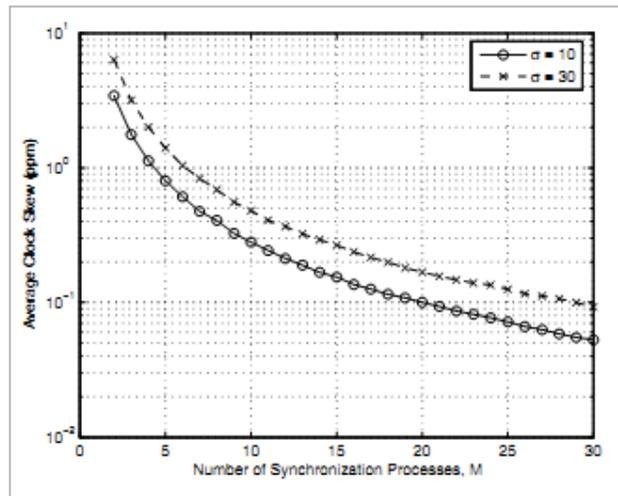
Fig. 6: Average clock skew in different receive delay difference standard deviation,  $\sigma$  [8].
