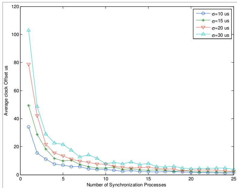
Fig. 11: Average clock offset on different receive delay difference in standard deviation for 50 nodes.
