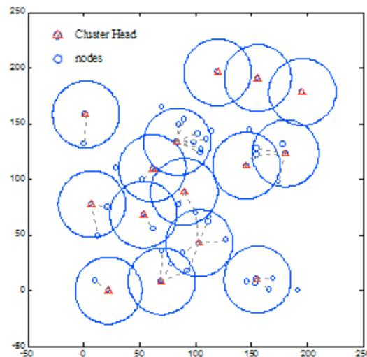
Fig. 10: Cluster head section and cluster formation for 50 nodes.
