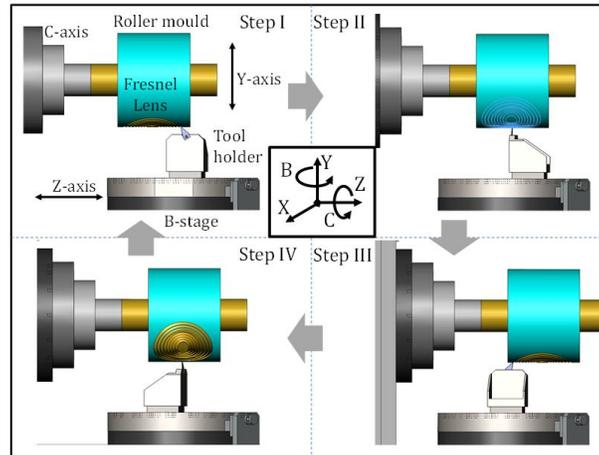
Fig. 25: 4-Axis integrated tool-work piece motion [40].
