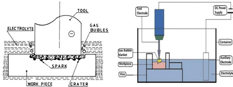
Fig. 19: Material removal mechanism of ECDM process (left) [28]; Schematic of ECDM process (right) [29].
