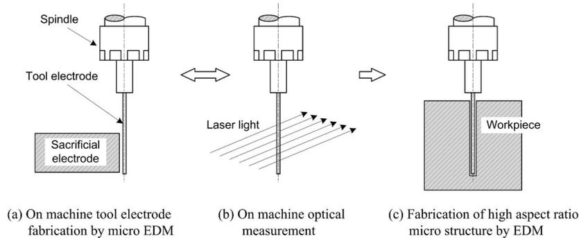
Fig. 5: Micro-EDM with on-machine-tool fabrication and on-machine-tool inspection steps in Mikrottools DT – 110 machine [8].
