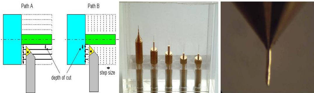
Fig. 8: (a) Two possible ways to do turning; (b) Micro shafts of diameter 50 microns; (c) Bending of micro shafts in conventional turning below 50 microns [13].
