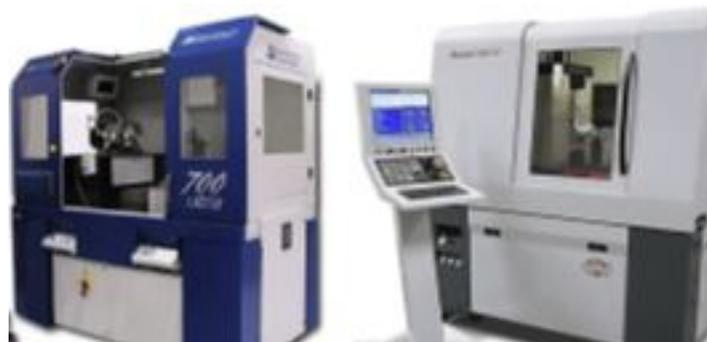
Fig. 6: Examples of multi-axis diamond turning machines: Nanoform 700 Ultra (left) [10], and Nanotech 350FG (right) [11].
