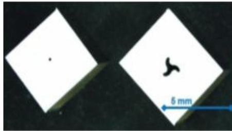
Fig. 14: Optical image of a pattern for micro punching (right) fabricated via micro wire EDM from a high-precision micro deep hole (left) drilled using a parylene-C-insulated tool electrode [18].
