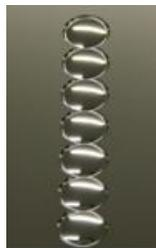
Fig. 22: Micro-lens array pattern generated by diamond micro milling of each lens individually [37].
