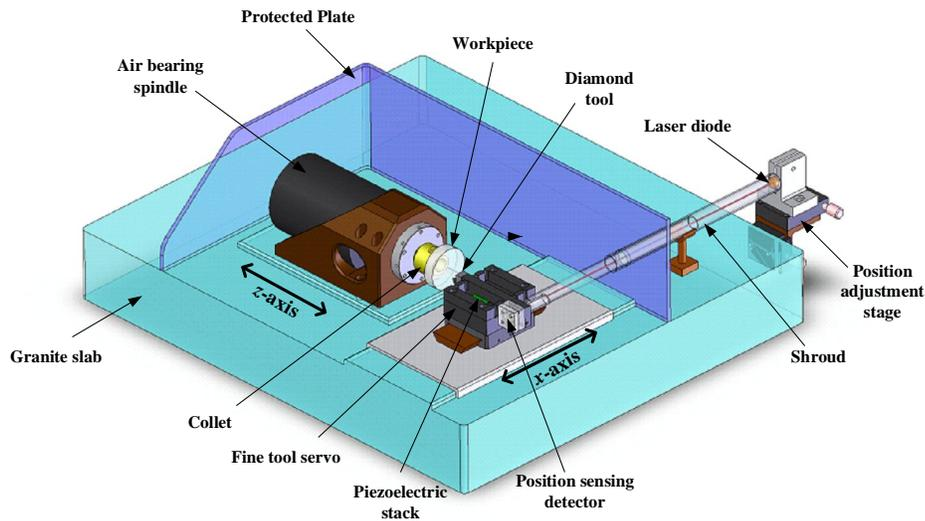
Fig. 7: FTS-High speed diamond turning machine (UPL –Series) [12].
