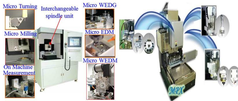
Fig. 4: Integrated multi-process machine tool from Mikrottools (left); multiple function machine from Takashima (right) [6, 7].
