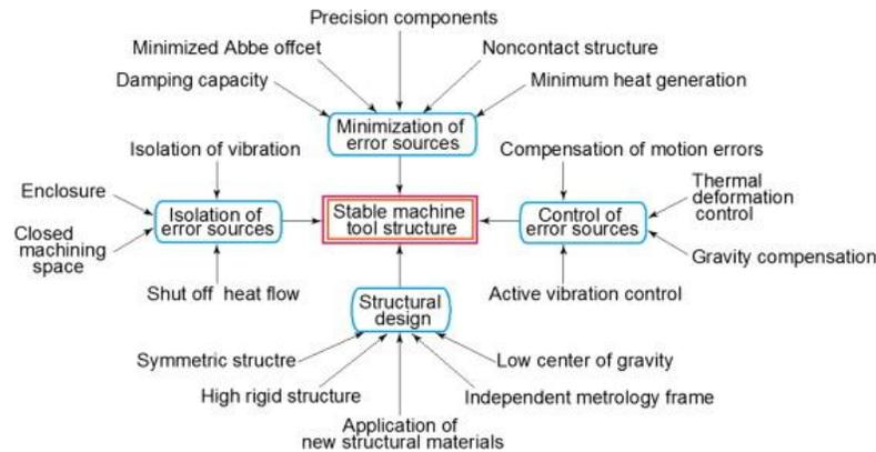
Fig. 1: Concept of stable mechanical tool structure for micro and nanometer-scale processing [3].
