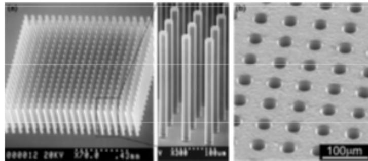
Fig. 16: (a) A  $20 \times 20$  array of LIGA-fabricated copper electrodes; (b) through-holes batch-machined in 50 mm thick stainless steel by the micro-EDM process using the array of electrodes shown in (a) [20].
