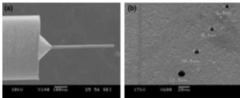
Fig. 11: (a) A 19-mm graphite electrode of 0.5 mm length fabricated by a micro-EDG–micro-turning compound process; (b) micro holes (up to 6.5  $\mu\text{m}$  hole in 50  $\mu\text{m}$  plate) fabricated with the microelectrode obtained by the micro-turning–micro-EDM drilling compound process [6].
