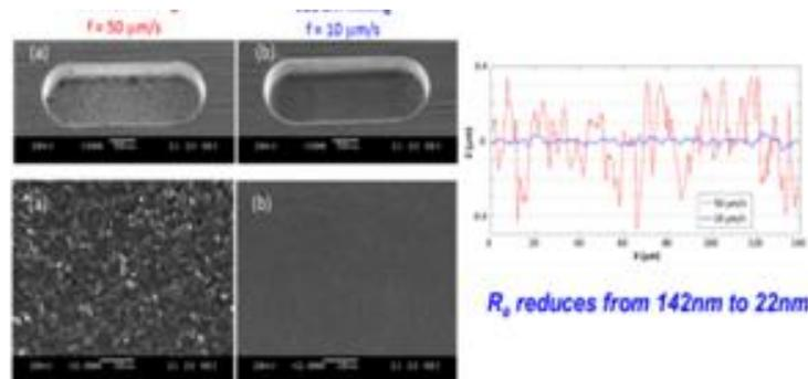
Fig. 17: Simultaneous EDM and ECM (SEDCM) process carried out in each cycle (EDM during on-time and ECM during off-time) to improve the surface finish to mirror finish (Machine Model: DT – 110) [21].
