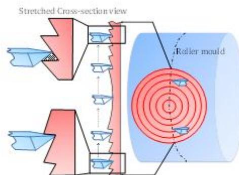
Fig. 24: Inability of the ultra-precision diamond turning method to machine a radial Fresnel lens on a roller [40].
