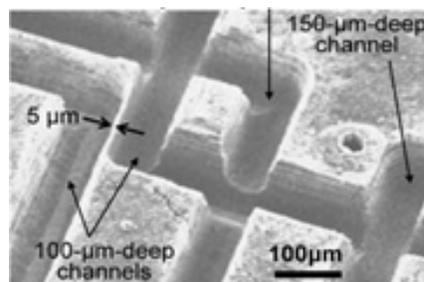
Fig. 9: Multi-level micro channel structures patterned in a CNT forest using micro-EDM [14].
