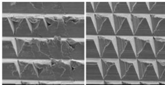
Fig. 20: Comparisons of pyramid patterns machined by conventional cutting (left) and elliptical-vibration cutting (right) (work piece material: Inconel 600) [30].
