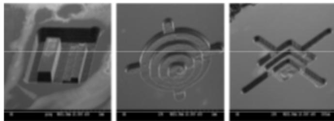
Fig. 18: Examples of 3D microstructure pattern in Pyrex glass [27].
