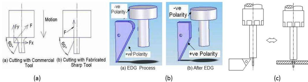
Fig. 10: (a) Modification of a conventional cutting tool using the micro-EDG (variant of micro-EDM) process; (b) a schematic representing the compound process combining modification of a cutting tool by micro-EDM and turning of a micro shaft by a modified tool tip; (c) compound process of fabricating a microelectrode using micro turning and applying a fabricated microelectrode in the micro-EDM drilling [16].
